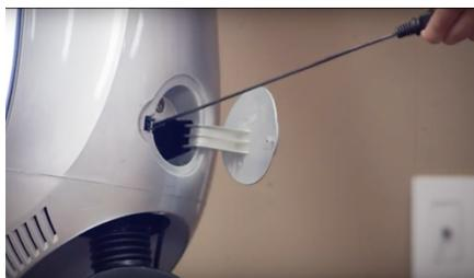
**Charging the Ojo:** A patented on-board charger with hidden cord plug behind a door on the front of the scooter, allows commuters to charge the Ojo in a standard (110v) wall outlet. Additionally, it is equipped with a state-of-the-art best in breed lithium ion battery featuring the highest quality lithium cell technology, ensuring riders the best performance each time.
