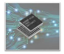
The AWMF-0139 operates at 24.25 GHz to 27.5 GHz, supports 4 radiating elements, and includes gain and phase controls for analog RF beam steering. Anokiwave's patent-pending IP blocks implemented in silicon technology enable low-cost hybrid beam forming with high energy efficiency and 5G fast beam steering<sup>tm</sup>.
